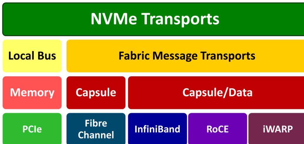
When sending complex messages to an NVMe over Fabrics device, the capsules allow multiple small messages to be sent as one message, which improves the efficiency of the transmission and reduces latency. The capsule is either a submission queue entry or a completion queue entry combined with some amount of data, metadata or Scatter-Gather Lists (SGLs). The content of the elements is the same as local NVMe protocol, but the capsule is a way to package them together for improved efficiency.
